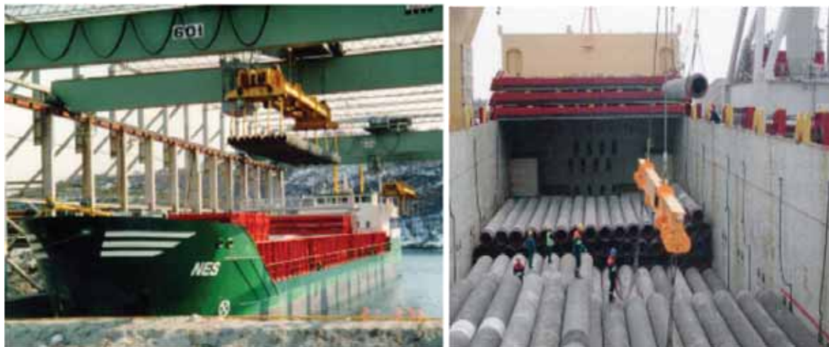
Figure 4-15. Loading coated pipe joints onto the pipe-supply vessel. (Photos by Nord Stream AG)
