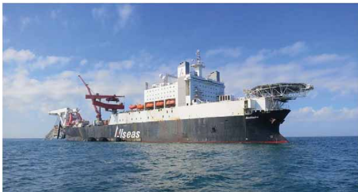
Figure 4-13. Typical DP Vessel – Allseas Solitaire.
