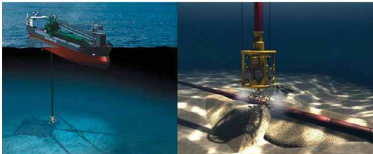
Figure 4-8. Rock placement on the seabed through a fallpipe. (Drawing by Nord Stream AG)
