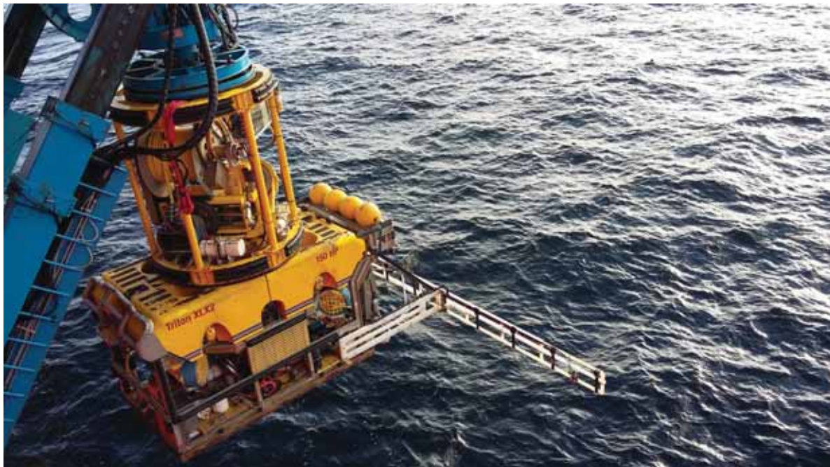
Figure 4-6. Remotely operated vehicle (ROV) equipped with a gradiometer. Photo by Nord Stream 2 AG.
