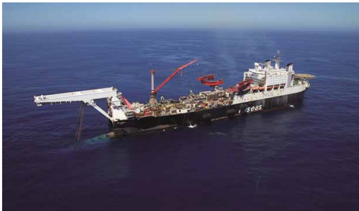
Figure 4-10. The S-lay pipe-lay vessel and survey support vessels.
