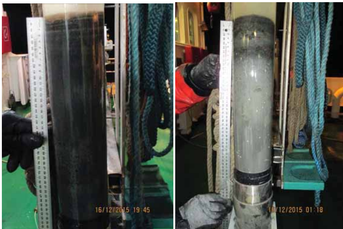
Figure 7-6. Sediment profiles at areal stations FIN_EBS_LUO_5 and 7 (Figure 7-7). Water depth was 71 m (left image) and 111 m (right image).
