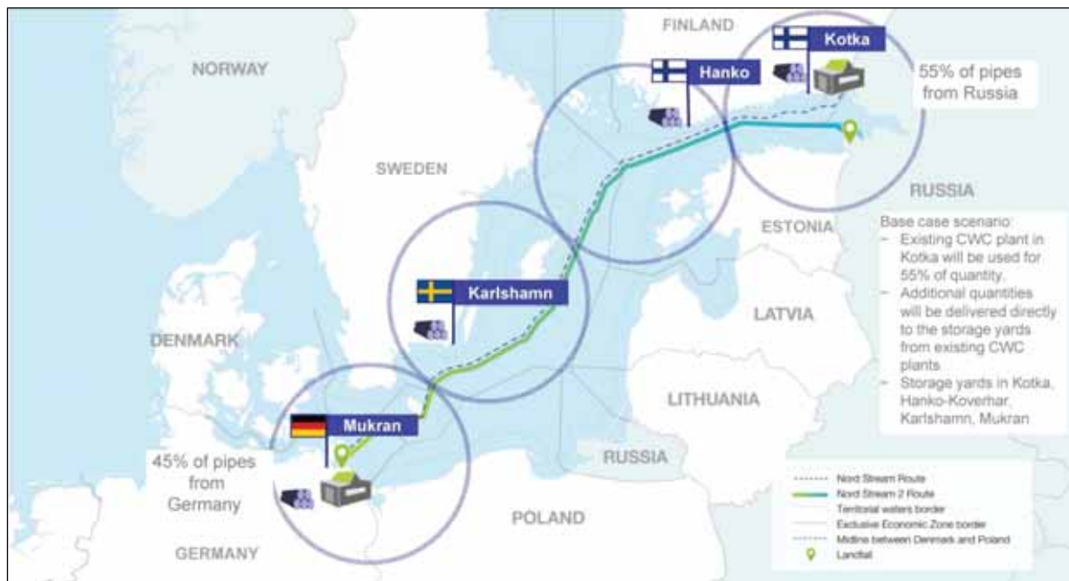
Figure 4-14. Pipe joint logistics Nord Stream 2.
