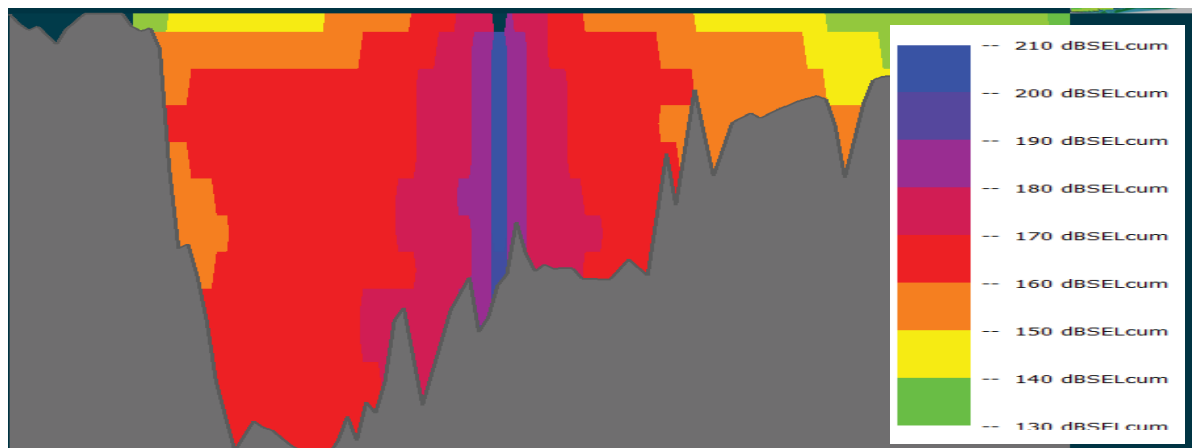
Figure 11-21. Explanatory figure showing how underwater noise propagates more efficiently in the deep waters than at the surface. Examples of vertical plot of munitions clearance sound propagation (colour scale) vs. depth (Y axis, 80 m) and distance (X axis, 50 km). Figure taken from underwater noise report (Ramboll 2016d).
