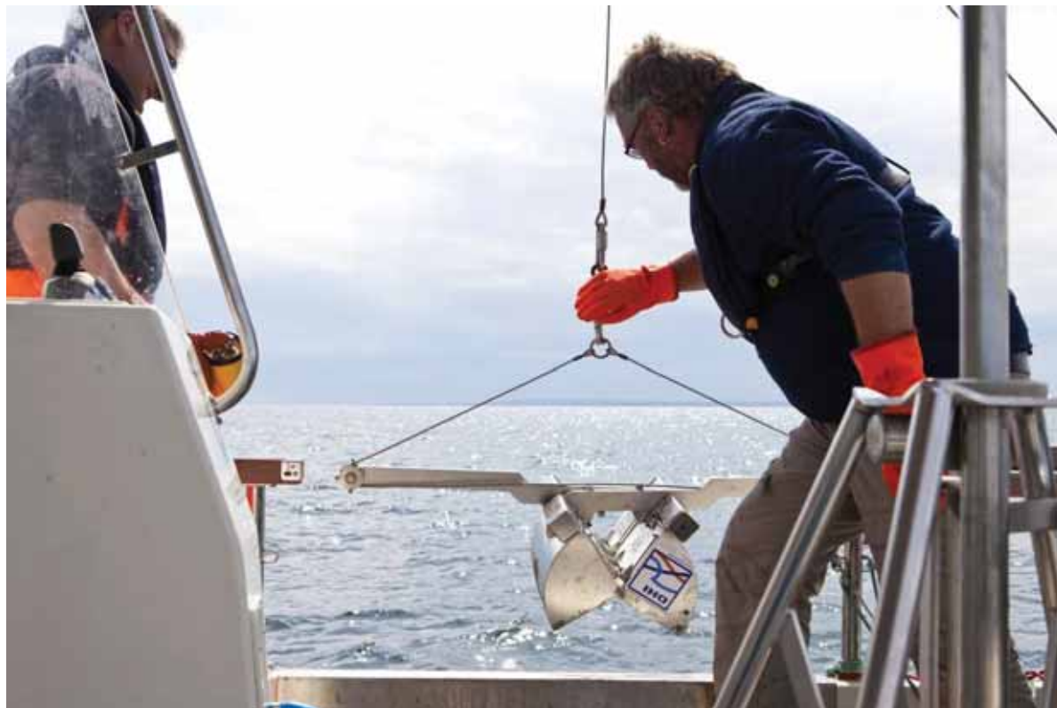
Figure 4-21. Van Veen sampler used in benthos sampling. Photo by Nord Stream AG.
