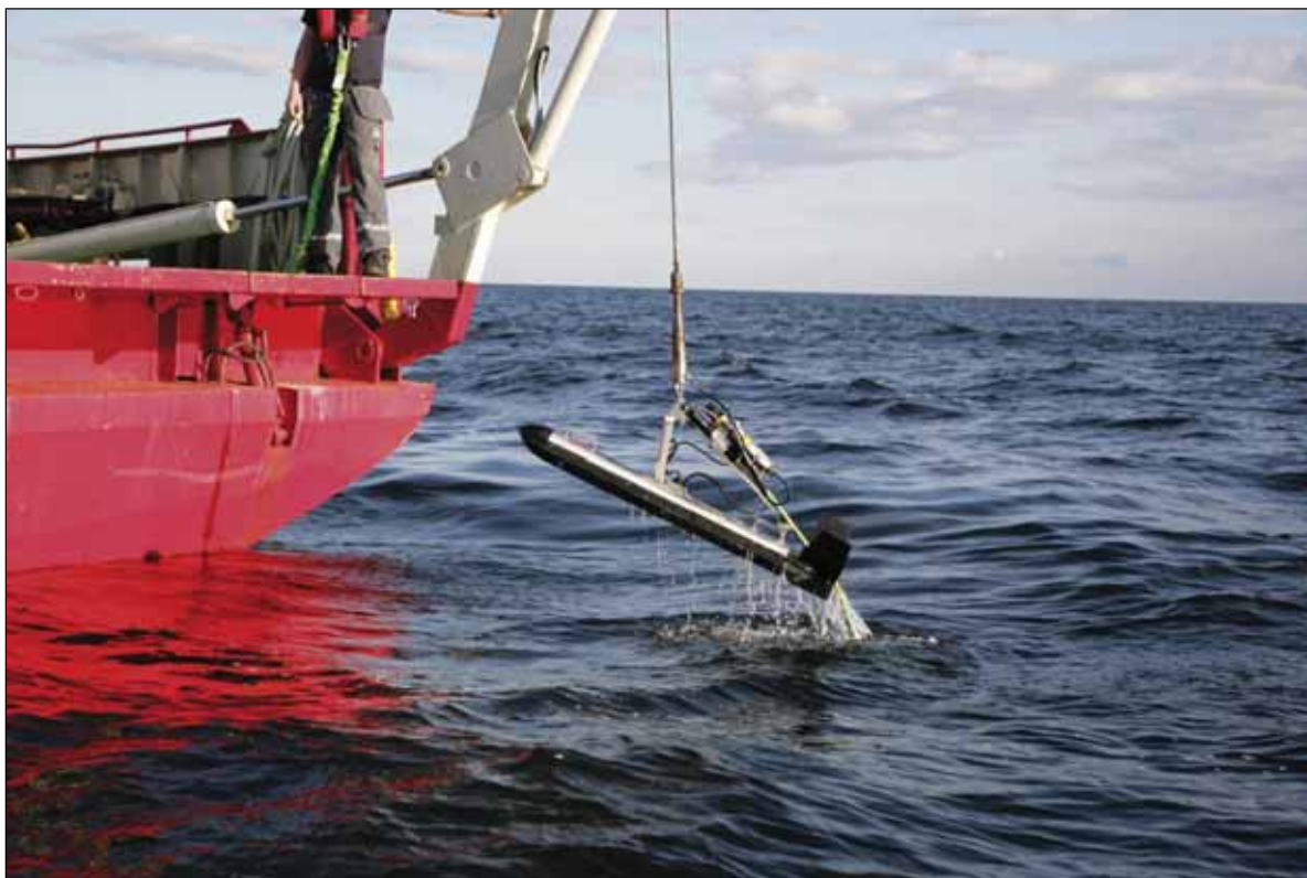
Figure 4-5. Side scan sonar (SSS) used in geophysical surveys. Photo by Nord Stream AG.
