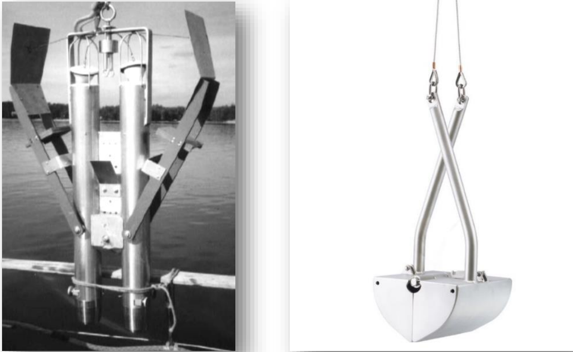
Figure 13. GEMAX sediment sampler (left) and Van Veen benthos sampler (right).
