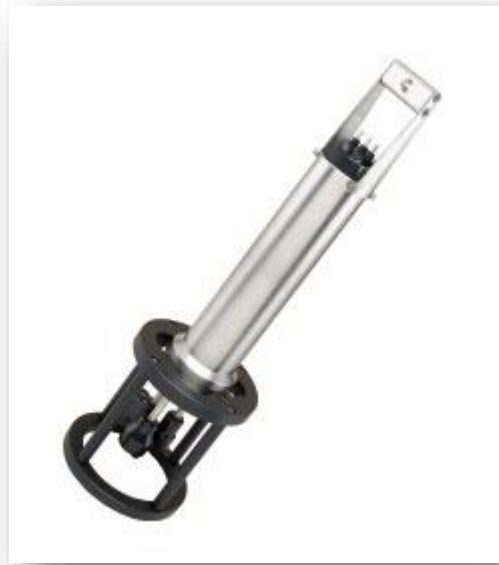
Figure 12. Rinko CTD -profiler for vertical profiling of salinity, temperature, depth, turbidity and dissolved oxygen concentration.
