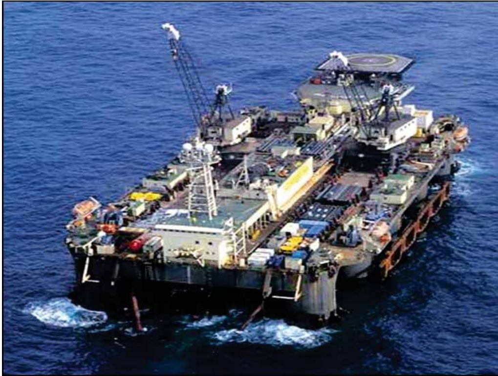
Figure 6-13 Castoro-Sei pipe-laying vessel.
