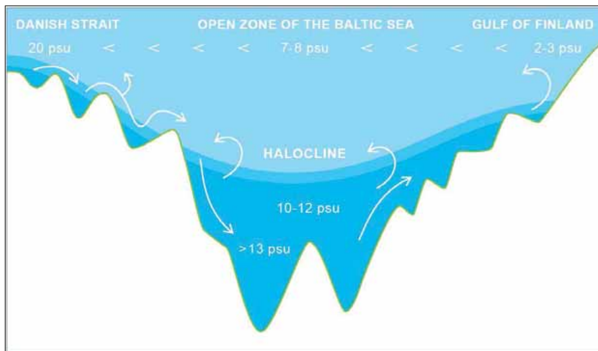
Figure 9-6 The heavy, saline water flows along the bottom, and the less saline surface water flows out of the Baltic Sea. The water becomes stratified, and a halocline separates the layers of varying salinity /63/.
