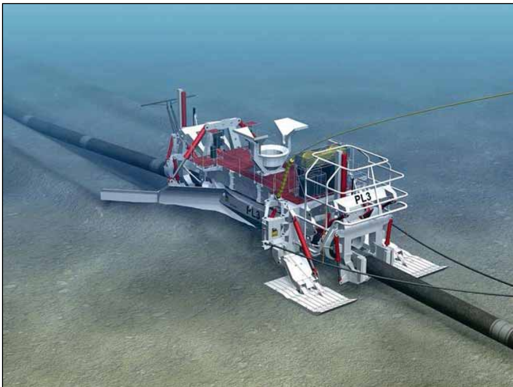
Figure 6-15 Pipeline plough in operation on the seabed.
