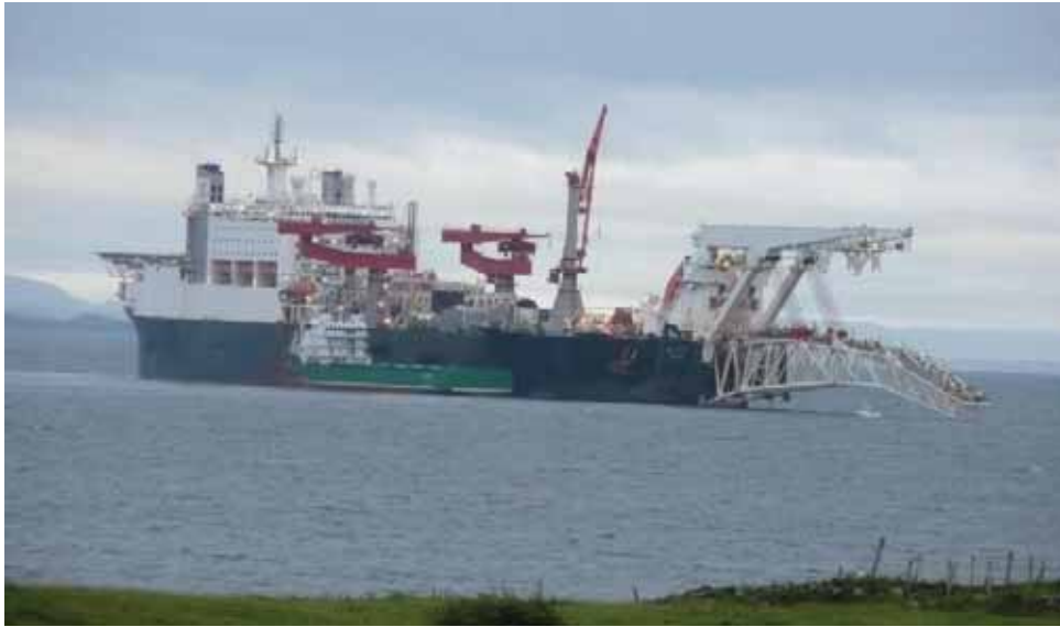
Figure 2-2 The lay barge Solitaire used in the Gulf of Finland.
