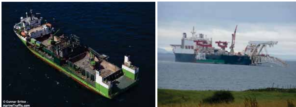
Figure 4-5 Left: the rock placement vessel Tideway Rollystone . Right: the lay barge Solitaire used in the Gulf of Finland.
