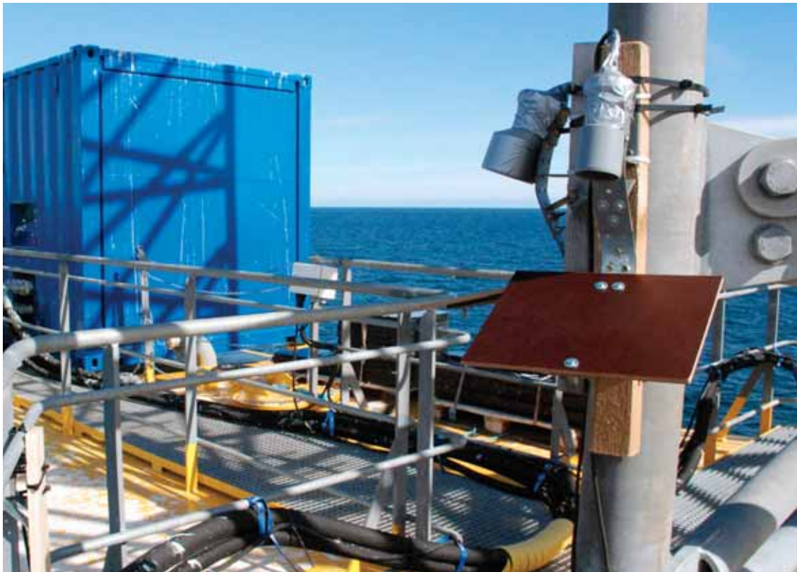
Figure 5. Microphones that gathered sound from above. The sound bounces off the reflector plate into the microphone. This is a tried and tested technique. Photography: Petra Bach.
