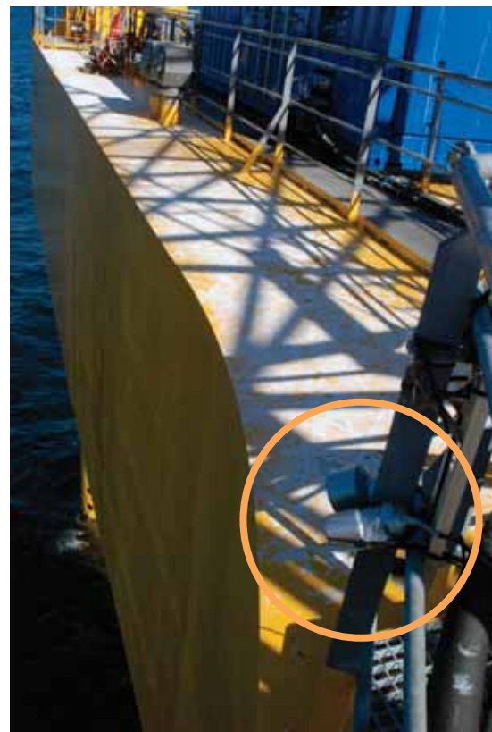
Figure 4. Picture of the Avisoft and Anabat microphones that have gathered sound from below, i.e. at a height of < 24 metres. Photography: Petra Bach.
