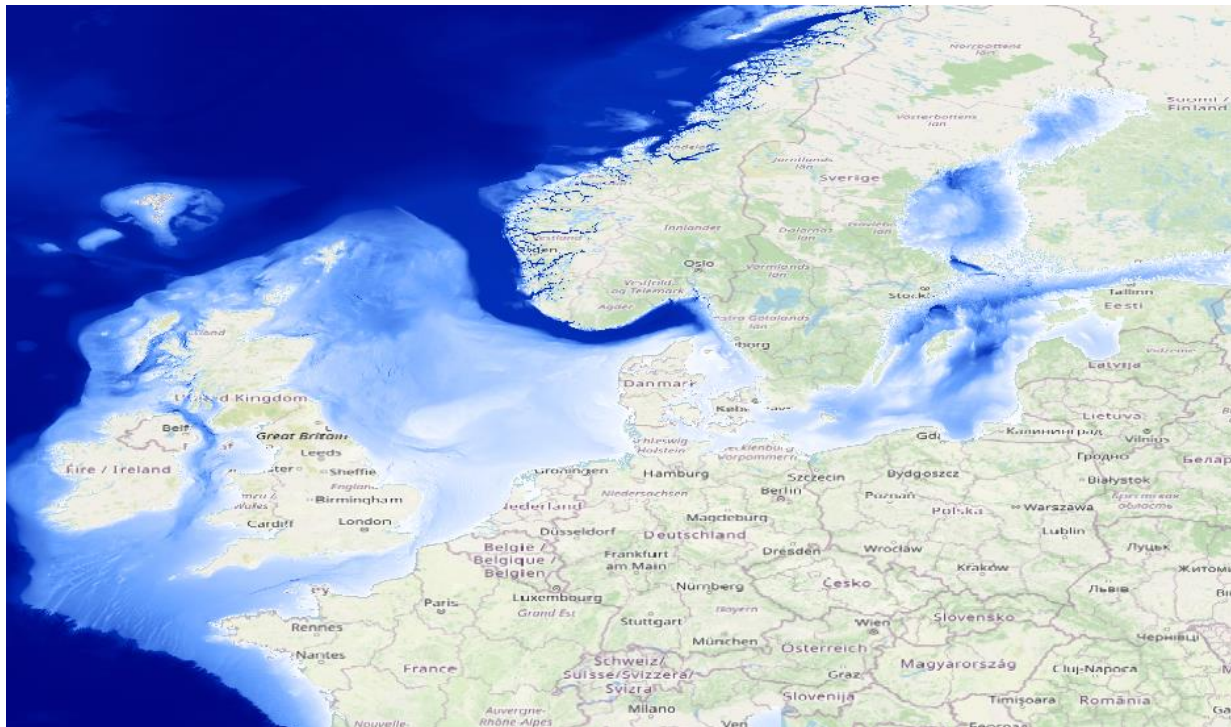
Figure 6.7: Bathymetry map over European waters from EMODnet, where light blue indicates shallow waters and dark blue indicates deeper waters (EMODnet, 2021).
