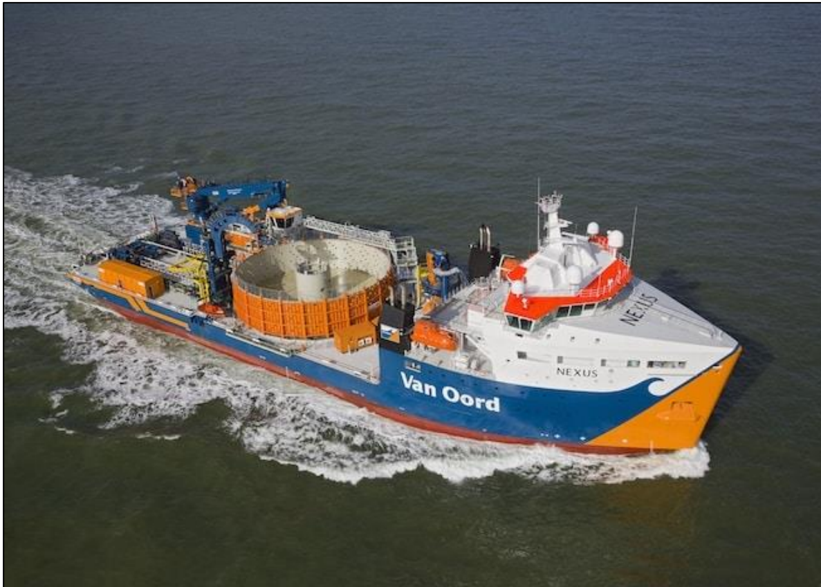
Photograph 2. Cable laying vessel
