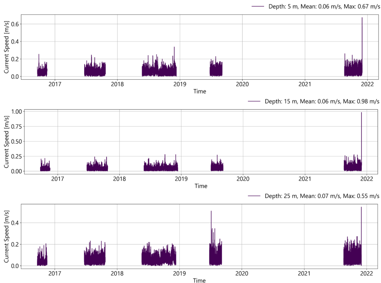
Figure 6.5: Measured current speed at NORRBYN at 5 m, 15 m, and 25 m depth (from top to bottom).
