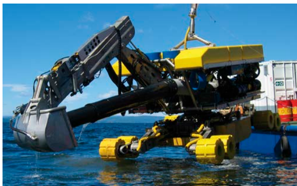
Figure 3-6. Dredging techniques. Shown above is a remotely operated “spider” and below a dredging barge and loading vessel (Ramboll 2014a).
