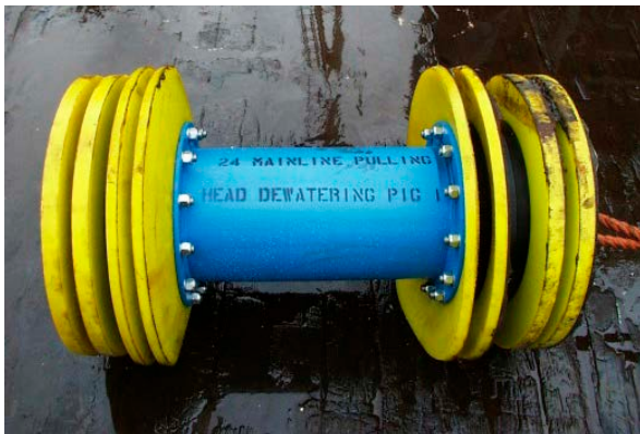
Figure 3-22. A typical de-watering pig (Ramboll a).
