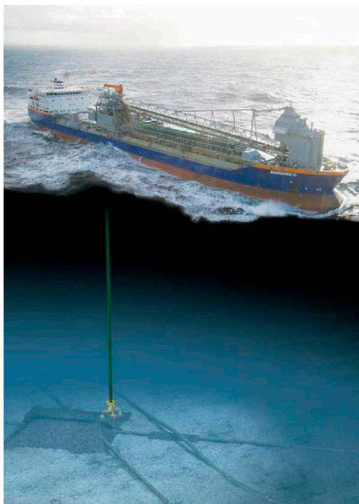
Figure 3-8. Subsea rock installation - accurate positioning by fall pipe. (Ramboll 2013)
