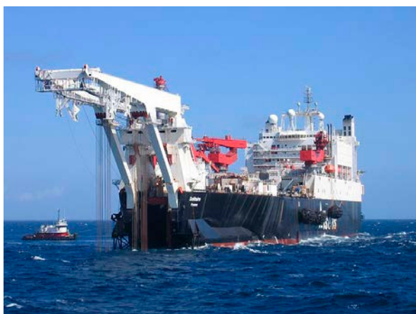
Figure 3-12. Typical pipelaying vessels – a dynamically positioned pipelaying vessel ( Solitaire , left) and anchored pipelaying vessel ( Castoro Sei , right). ( Ramboll 2013a )
