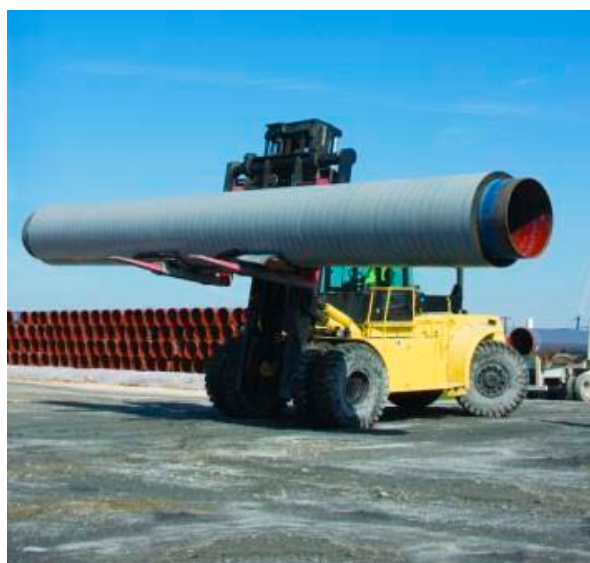
Figure 3-2. Line pipe with a (black) polyethylene coating inside a concrete coating. (Ramboll 2013aa)
